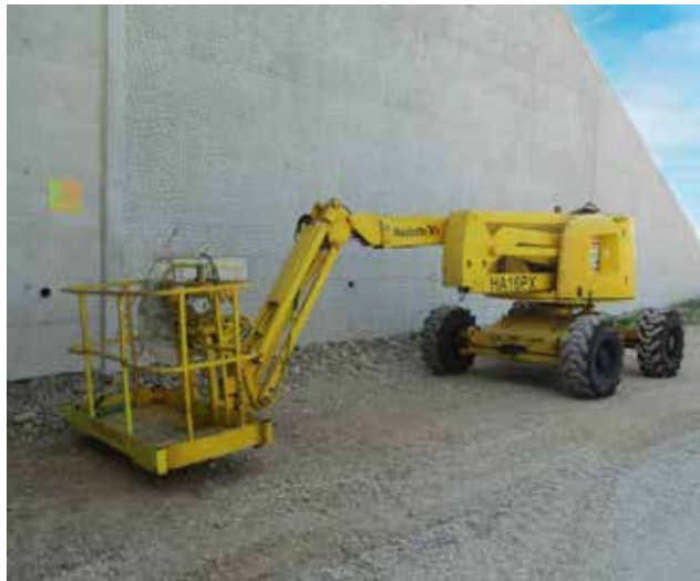
Nacelle positive automotrice
